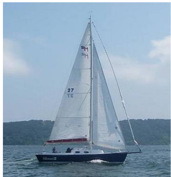
Note the stack pack for the main and the Rollgen gennaker furling system. These items were added during the commissioning of the boat.
