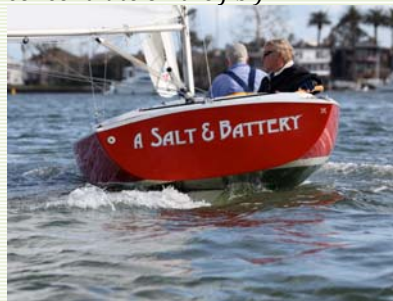
Really slow! (Jim is turning around the mark with the tiller clear to weather. The rudder isn't steering any more – it is just stopping the boat.)
